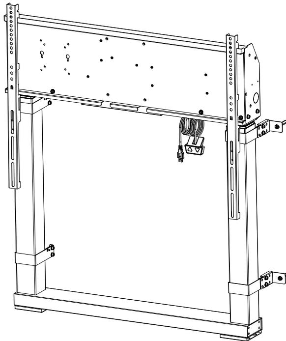
For using this product properly and safely, please follow the Installation and Operation Manual. It is suggested that this Electric Stand applies to the 55-86 inch interactive Large Format Display. Use with other equipment may result in instability causing injury. This stand can carry a maximum weight of 120KG.
